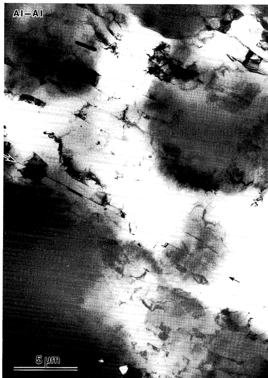
Fig. 4 A HVEM bright-field image of the interface of an Al-Al joint.
